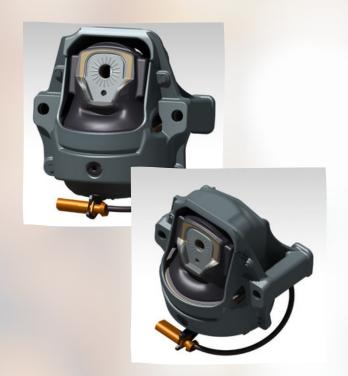
The electronic hydro-mount represents an innovative and enhanced version of the conventional hydraulic mounts. This type of hydraulic mounts is controlled by the vehicle ECU, through an actuator, , the mount's dampening capacity can be altered depending on the vibrationcaused by the engine.
