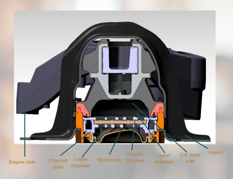
As you can see the mount is connected to the engine and with the car chassis. The pressure coming from the engine causes the engine mount to deform and make the fluid come down and up through the two chambers, and this motion of the fluid absorbs most of the vibration energy. An internal valve is designed to change the route of the fluid depending on the vibration frequency, hence yielding a more comfortable ride and longer mount life.
