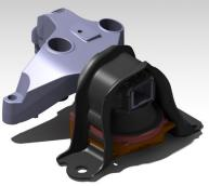
Hydraulic engine mounts on the other hand have a hydraulic fluid (water & glycol) inside of them and are characterized by a dampening capacity that is superior to that of the solid or elastomeric engine mounts.
